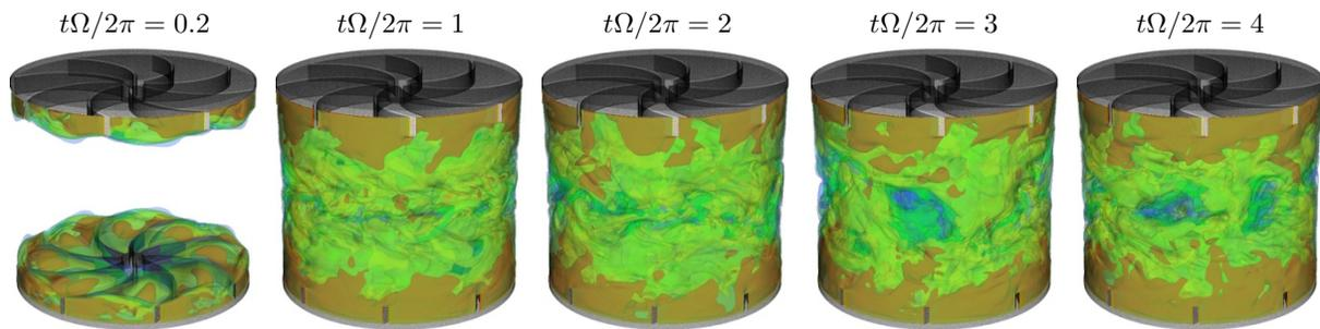
Figure 2 - Iso-surfaces of velocity in the von Karman device
