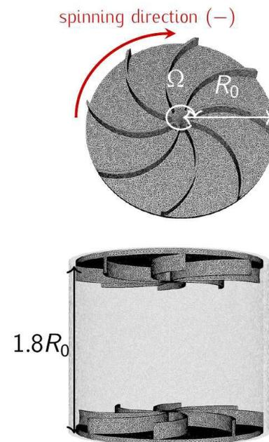
Figure 1 - Schematic of the von Karman device.
