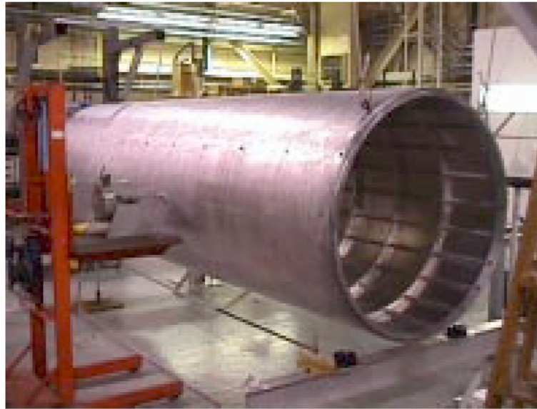
Fig. 40. NASA Aluminum Testbed Cylinder (ATC). Frame and skin.
