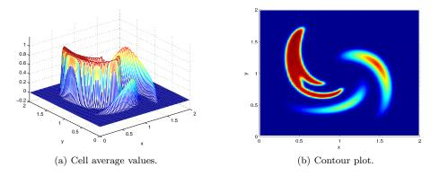
Fig. 7.11. Ex. 8. Second order Strang splitting solution at time t=0.75=T/2 using  $\Delta t=8h$  (CFL $_{\Delta t}=16$ ).
