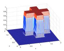
Fig. 7.2. Ex. 5 with an initial cross pattern. Plot of cell average values at t=0.5 using  $\Delta t=10.5h$ . The time step does not allows reproduction of the cross pattern on the grid.
