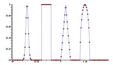
Fig. 6.1. Ex. 4. Shu's linear test with m=160. The blue curve shows the exact solution, while the solid black squares are the exact solution at the center of each cell. The red circles are the computed solution plotted at the center of each cell.
