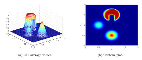
Fig. 7.9. Ex. 8. Second order Strang splitting solution at T=1.5 using  $\Delta t=12h$  (CFL $_{\Delta t}=24$ ).
