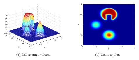
Fig. 7.7. Ex. 8. Second order Strang splitting solution at T=1.5 using  $\Delta t=4h$  (CFL $_{\Delta t}=8$ ).
