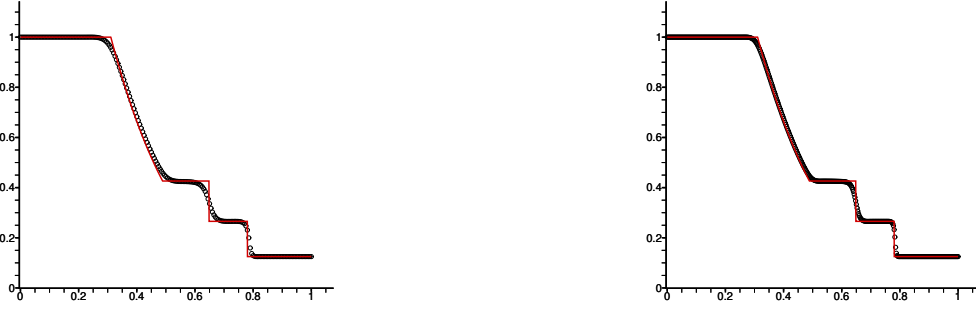
Figure 9: Ex. 5, Sod's 1-D shock tube test. The density profile at time T = 0.16 using \Delta t = 0.1h and m = 200 (left) and m = 400 (right) grid points.
