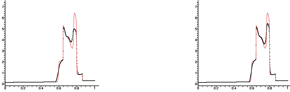
Figure 12: Ex. 6, Woodward and Colella's double blast test. The density profile at time T = 0.038 using m = 800 (left) and m = 1200 (right) grid points. The fine resolution reference solution is shown in red.
