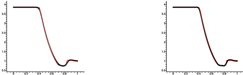
Figure 11: Ex. 5, Arora and Roe's Mach 3 shock tube test. The density profile at time T = 0.09 using \Delta t = 0.05h and m = 200 (left) and m = 400 (right) grid points.
