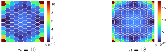
Fig. 9 The L^2 error on each element for mesh sequence \mathcal{T}_h^1 at level n = 10 and n = 18 with approximation index r = 5 .
