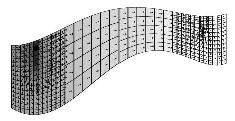
Figure 1: Computed pressure (shade) and velocity field (arrows) for the more practical example.
